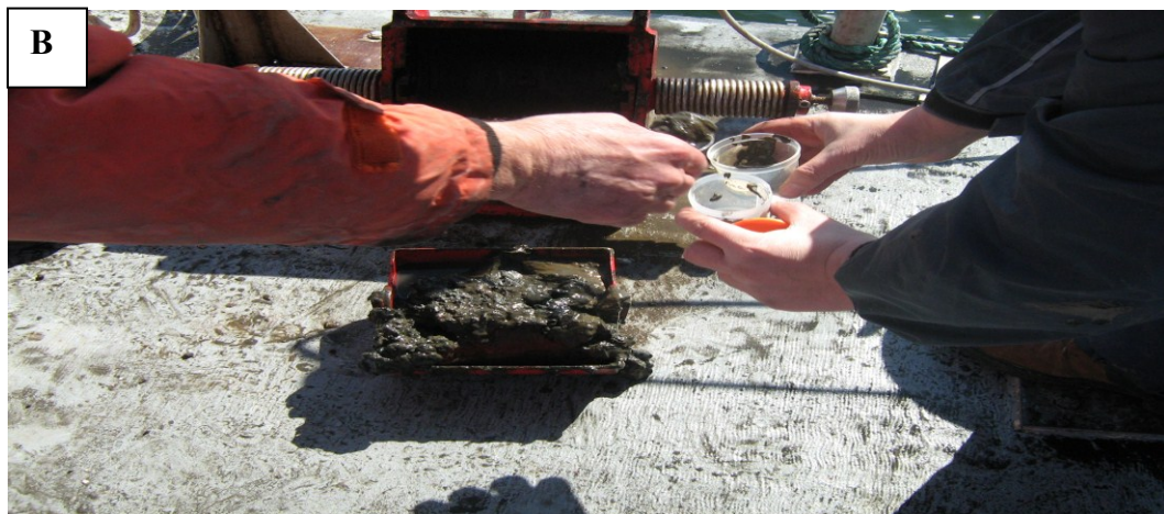
Figure 2.2: Photographs showing the sampling using a Shipek sampler: A. settling the sampler for opening after pulling it from the water; B. taking a sample from the upper few centimeters of the sampler and putting it in a vial for lab processing.
