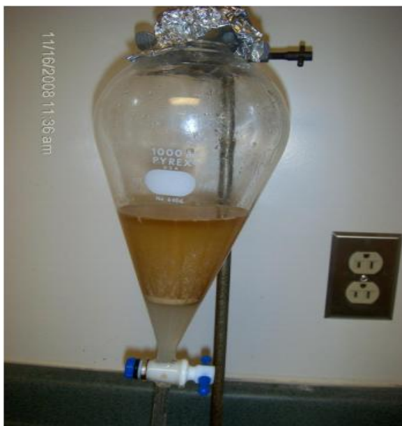
Figure 7.12 Soapnut biodiesel washing with warm distilled water
