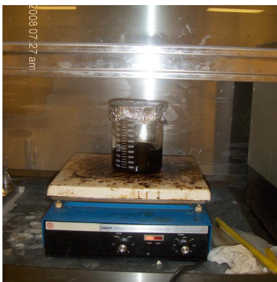
Figure 7.7 Batch transesterification process
