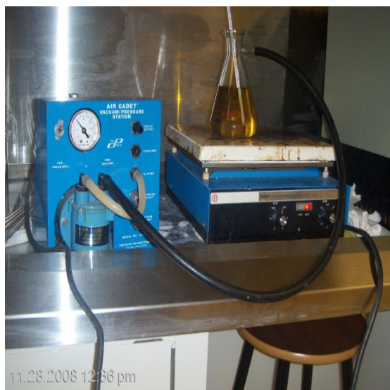
Figure 7.13 Removal of water by vacuum pump
