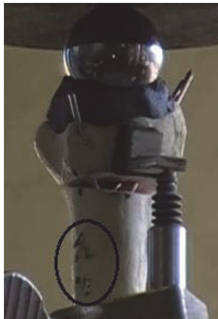
Figure 3.12: K-wire penetration through the medial cortex
