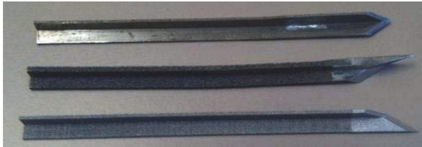
Figure 2.2: Implant prototypes (top: steel, middle: porous tantalum, bottom: porous titanium)
