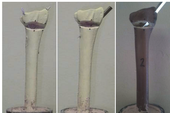
Figure 3.5: Implanted samples (left: FCS sawbone with k-wires, middle: FCS sawbone with implant, right: composite sawbone with implant)
