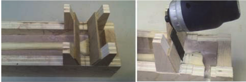
Figure 3.2: Custom cutting jig for creating fractures
