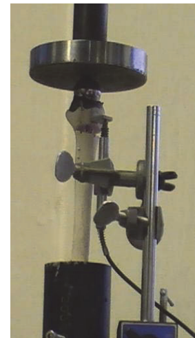
Figure 3.7: Experimental set-up of LVDT
