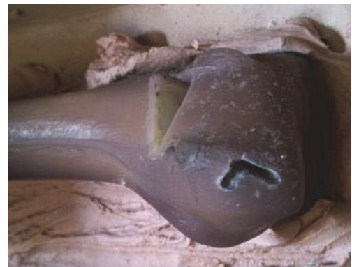
Figure 3.3: V-shaped slot in composite sawbone to permit implantation
