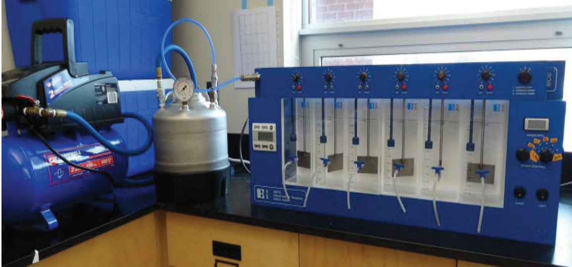
Figure 3.1. EC Engineering dissolved air flotation batch tester apparatus.
