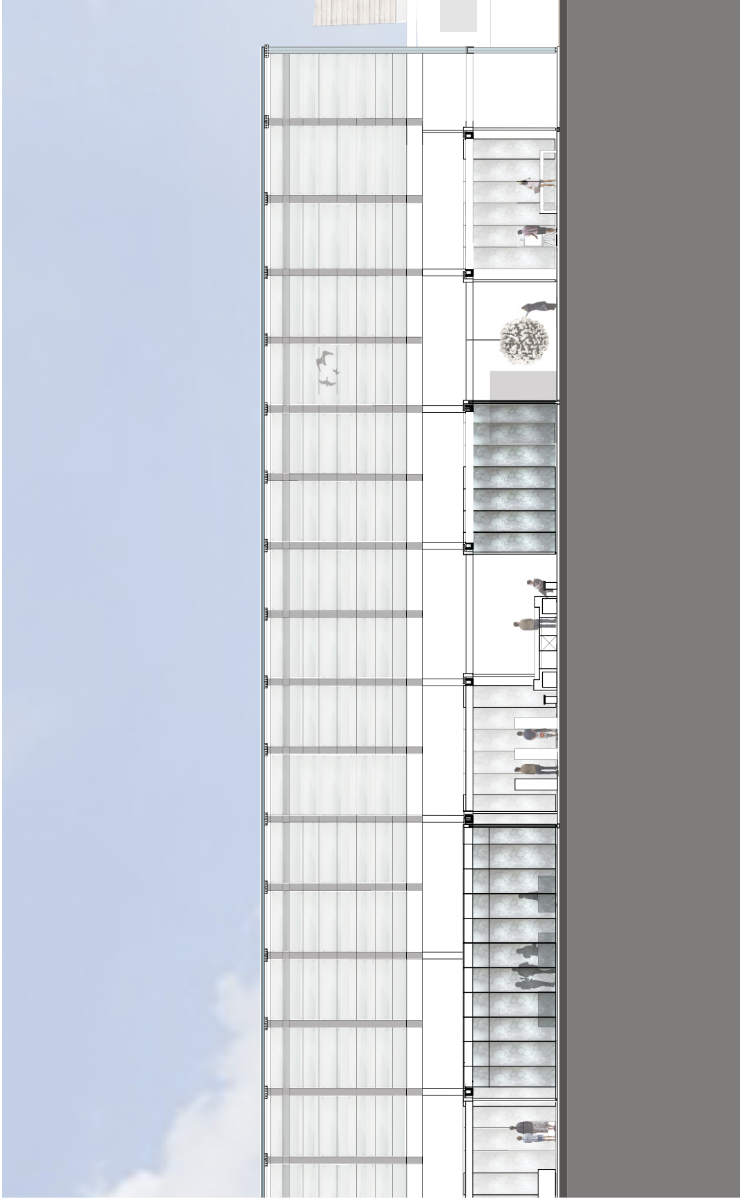
Long Section through exhibition and gathering spaces created by new glass roof and sliding stained-glass wall panel systems.
