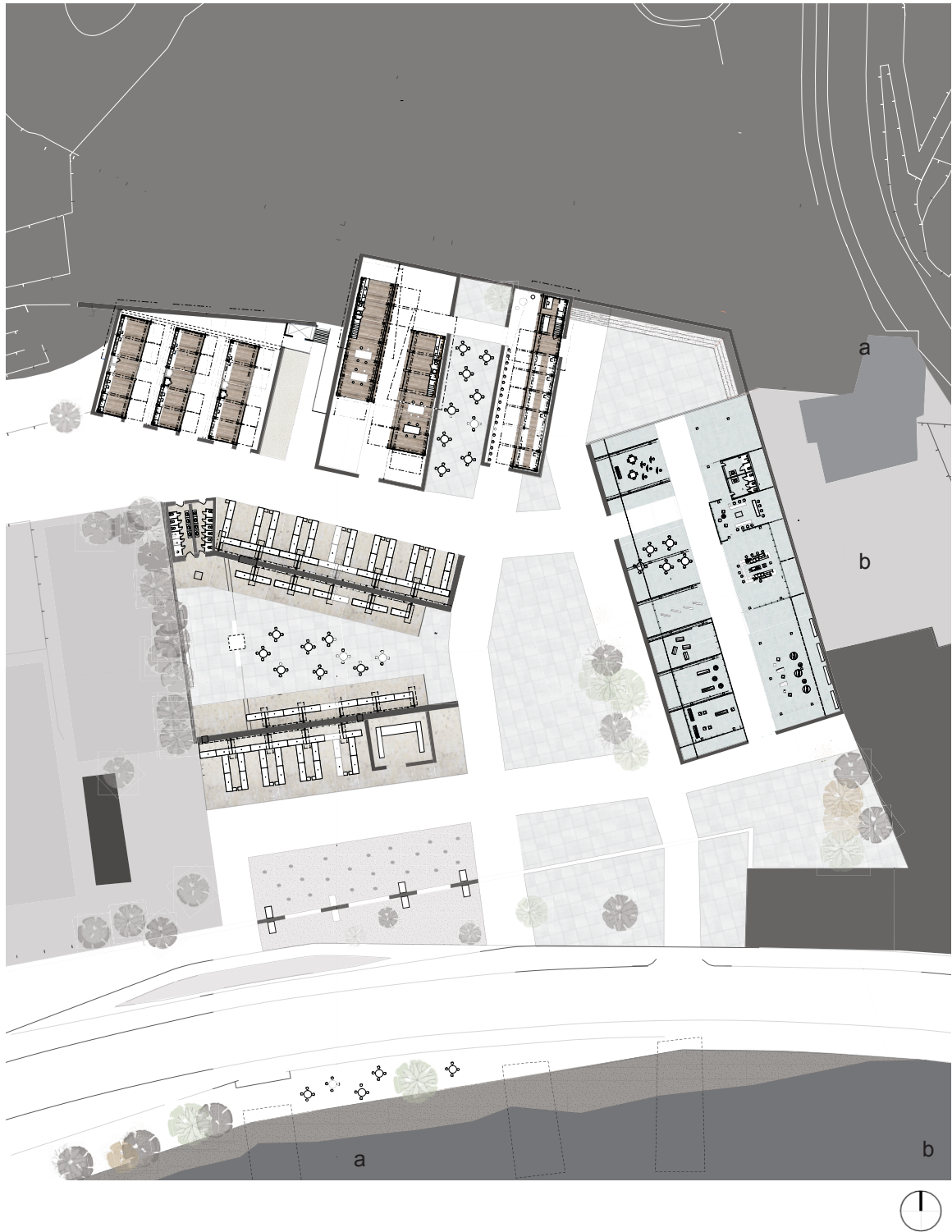
Ground level site plan showing the relationship between the public workshops, artists studios and food cart stalls (add) with art courtyards (mix, mark and fill) the exhibition and gathering space (insert and cover) and the outdoor market (expose and set out). The site is connected to the street.
