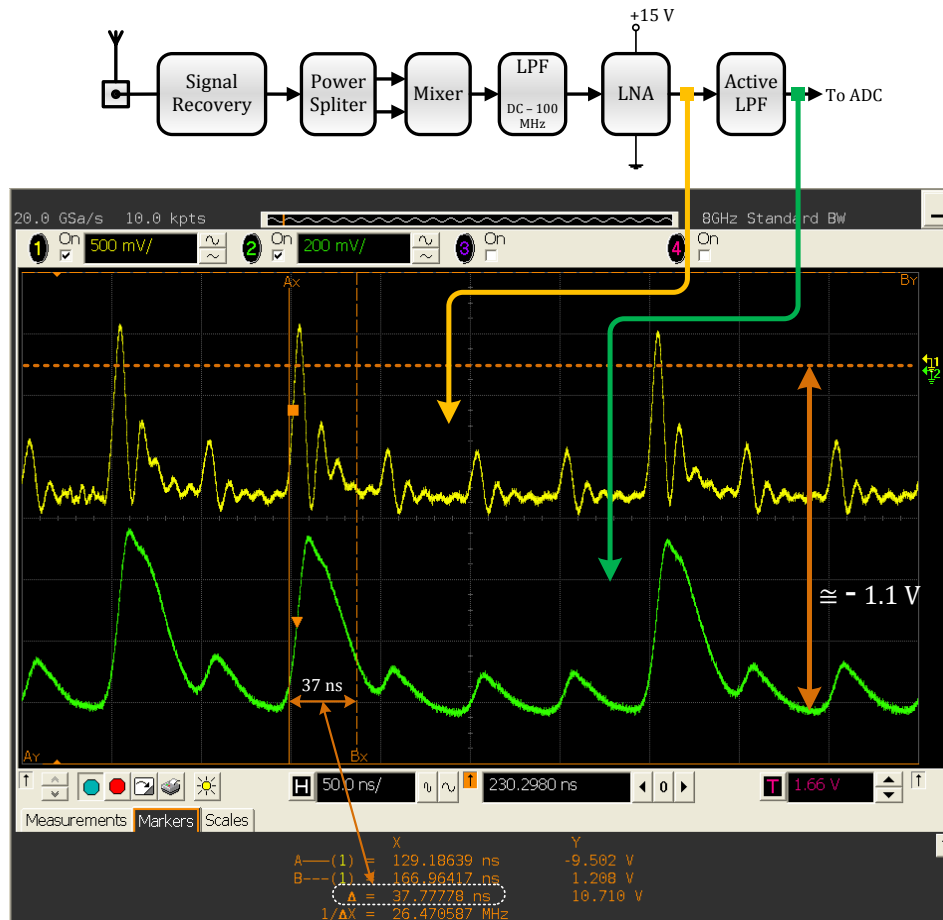
Figure 5.18: The implementation results before and after the two-pole active LPF circuit
