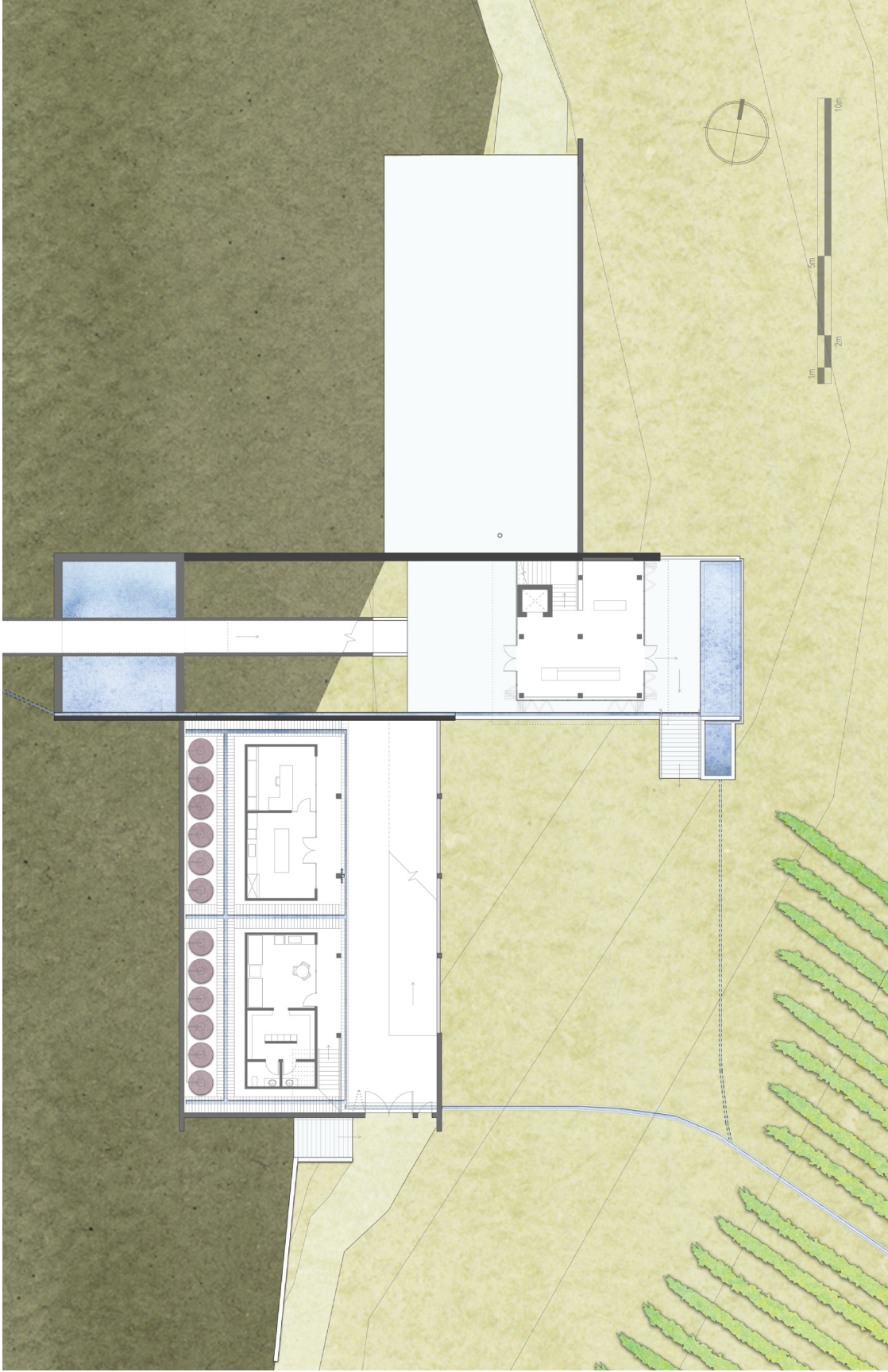
Level 2 Plan - Fermentation and Tasting Room. Purple shading marks fermentation tanks where grape juice transforms into wine.
