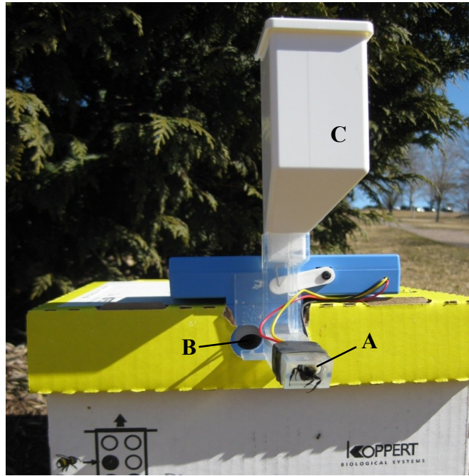
Figure 3.2. Koppert Biological Inc. top-loading mechanical biopesticide dispenser attached to a bumble bee hive for bee vectoring of biopesticides. (A) Dispenser exit tunnel wired with electronic sensor, and filled with biopesticide; (B) Return entrance to hive; (C) Top-loading reservoir for biopesticide, attached to gate mechanism and battery pack with electronics.
