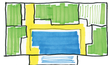
Space planing concept for “C” type big house. Green shows individual space, blue shared space, and yellow circulation.
