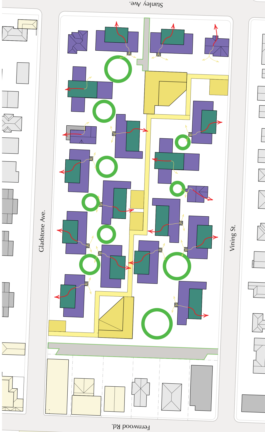
1:1000 plan diagram showing the proposal. Casual social interactions can happen in a variety of spaces, including back yards, the pedestrian street, front porches and the common houses, providing a very different social environment in the outdoor space than the existing conditions did.
