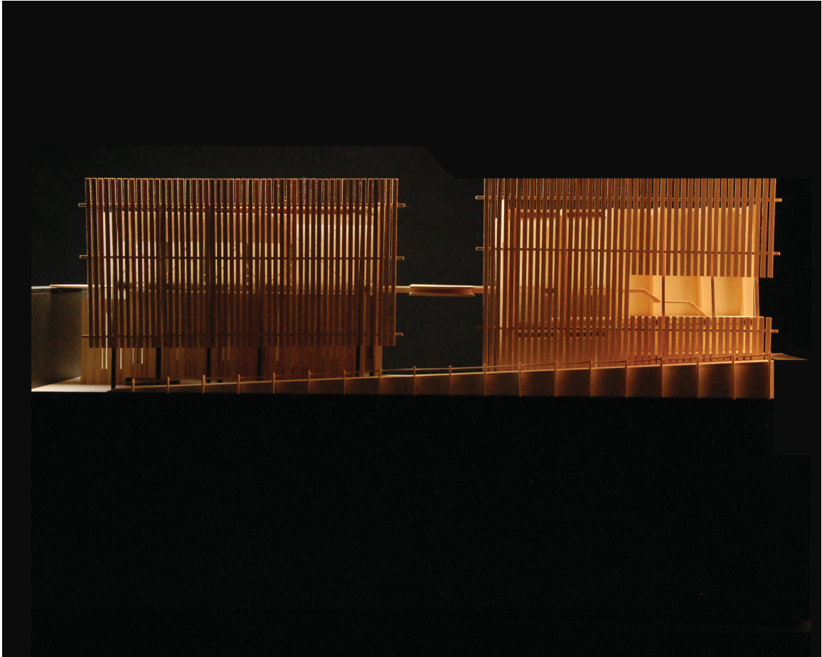
Presentation model, north elevation with screens to diffuse southern light.
