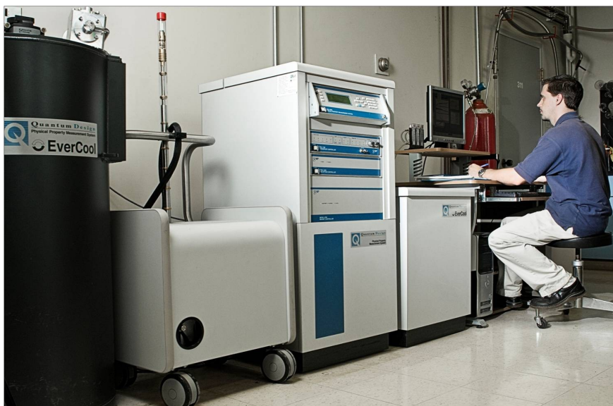
Figure 2.5: The Physical Property Measurement System. Components are, from left to right: Measurement chamber, ^3\text{He} probe, Computational hardware, User interface.
