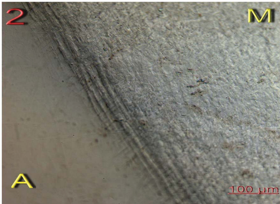
Figure 4.8 - Optical microscopy images of the microstructural evolution of superelastic TiNi during tensile testing while subjected to heating and cooling periods.
