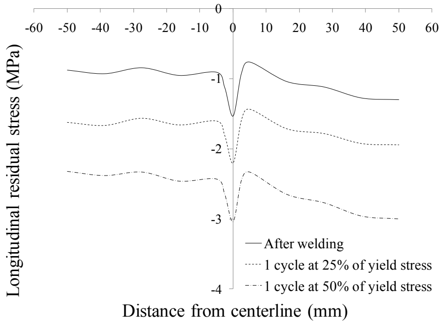
Figure 6.9, Longitudinal residual stress in flange of model T2
