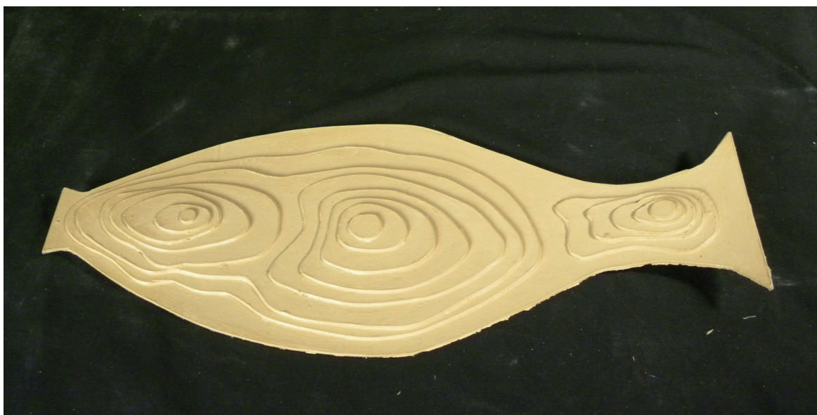
The ground counter line steps in the gathering hall. Each step is 25 cm in height.
