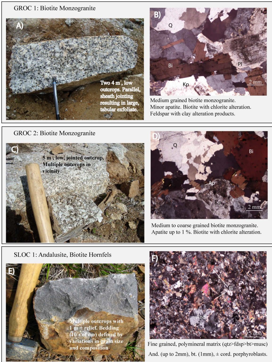
Figure 2.7: Field and petrographic photos (cross polarized light) of bedrock samples in Moose Pit Brook catchment. Q- quartz, Bi- biotite, Pl- plagioclase, Kp- potassium feldspar, Ap- apatite, And- andalusite.
