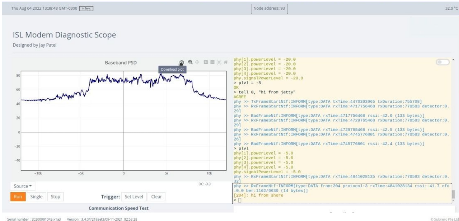
Figure 4.22: With the three nodes deployed at the COVE (4.16), a message was successfully relayed from the surface node (node # 3) to a submerged node (node # 2) via another submerged node (node # 1). Node # 1 as the relay node made the transmission possible as there was noLOS between the transmitting and intended receiving node. This relay mechanism enables communication over longer distances and enables better coverage in underwater acoustic networks. The successful message relay demonstrates the effectiveness and robustness of the communication system under the tested conditions.)
