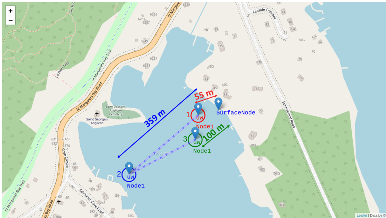
Figure 4.24: St. Margaret's Bay (uncontrolled environment) at 44.6802104 N, and 63.91634 W (farther from Halifax approaches) saw two underwater network nodes deployed. A surface underwater network node was deployed from the jetty and one submerged underwater network node was deployed at multiple stand-offs from the surface underwater network node. The one submerged underwater network node at 1, 2 and 3 was 55 m, 359 m and 100 m, respectively, from the surface underwater network node
