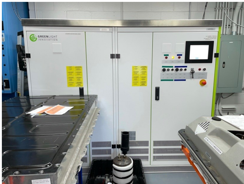
Figure 9: GLI-GK battery pack cycler
