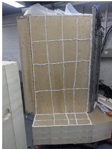
(e) Insulation glued to enclosure box
