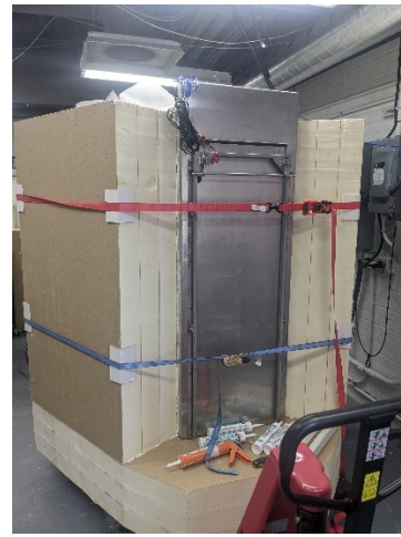
(f) Glued insulation held together using strap ties
