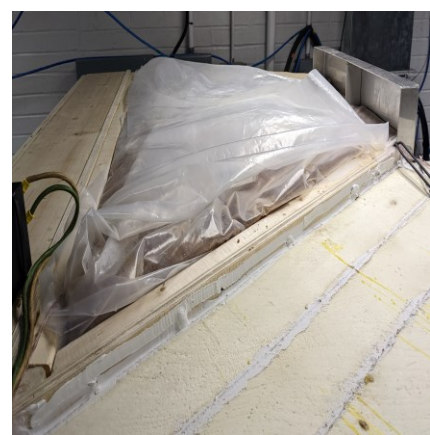
(i) Soil-filled test unit
