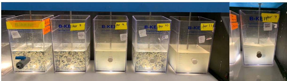
Figure 6.5: Visual Floc Characterization from Jar Tests (From Left to Right: Sample C, Sample A, f_{IA,0} = 0.1 , Sample B, f_{IA,0} = 0.2 , and the Control)
