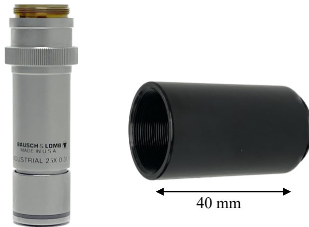
Figure 16 Left: photo of objective. Right: photo of 40 mm long C mount threaded tube.
