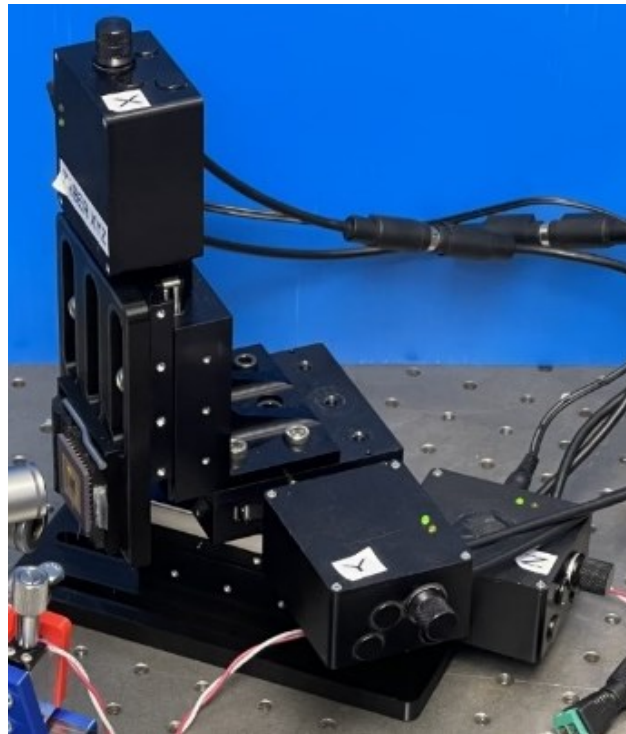
Figure 24 Zaber XYZ stage, table holes are 1” apart. XYZ letters refer to camera axes.
