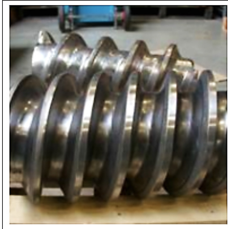
Figure 17. Pet-food granulate extrusion screws, coated with laser cladding, extended lifetime by ~300% [219].
