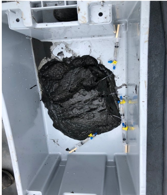
Figure 2.4: Sediment grab sample using rhizon samplers to extract pore water nutrients.
