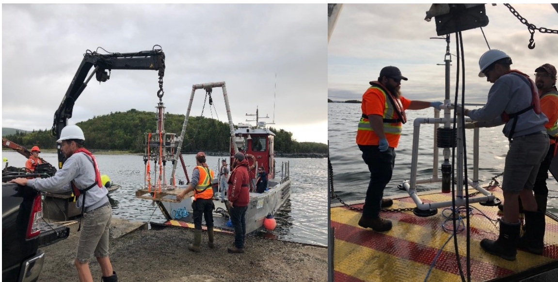
Figure 2.5: Left, a multi-corer being placed on the RV Gumby for use in 2019. Right, the hypoxic corer constructed in 2020 following the design of Gardner et. al, (2009).
