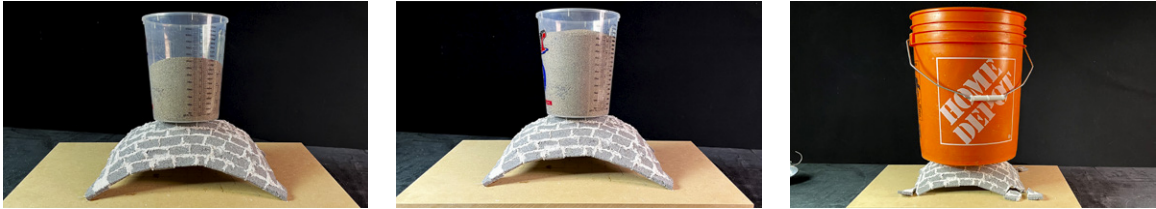
From left to right: 2kg load test, 3kg load test, and 6kg load test
