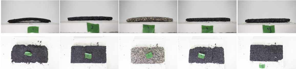
20cm x10cm x1.2cm tiles made with 5 different matrix dried at room temperature.
