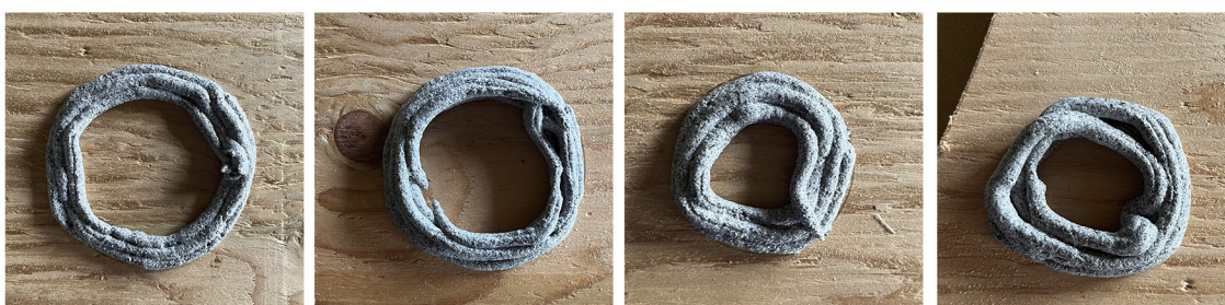
3-in diameter single wall, wall collapsed inward at third layer.
