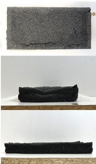
Preliminary 4in x 8in x 1in mould test
