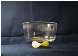
A single Pringle chip supports 175 times of its self weight through geometric equilibrium.
