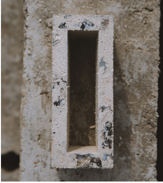
Fig. 53. Bio-bricks made from crushed shellfish shells (Howarth 2022).
