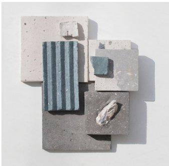
Fig. 34. Crushed seashells form a material with the hardness and texture of stone (Crook 2020).
