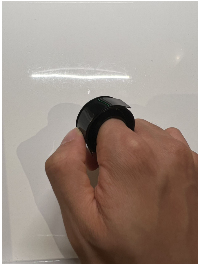
Figure 1.5: This is the first prototype device with a flexible touch-pad around the ring's surface.
