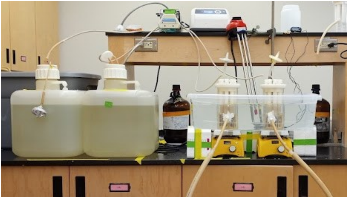
Figure 17. Set-up of CDC reactors on the bench
