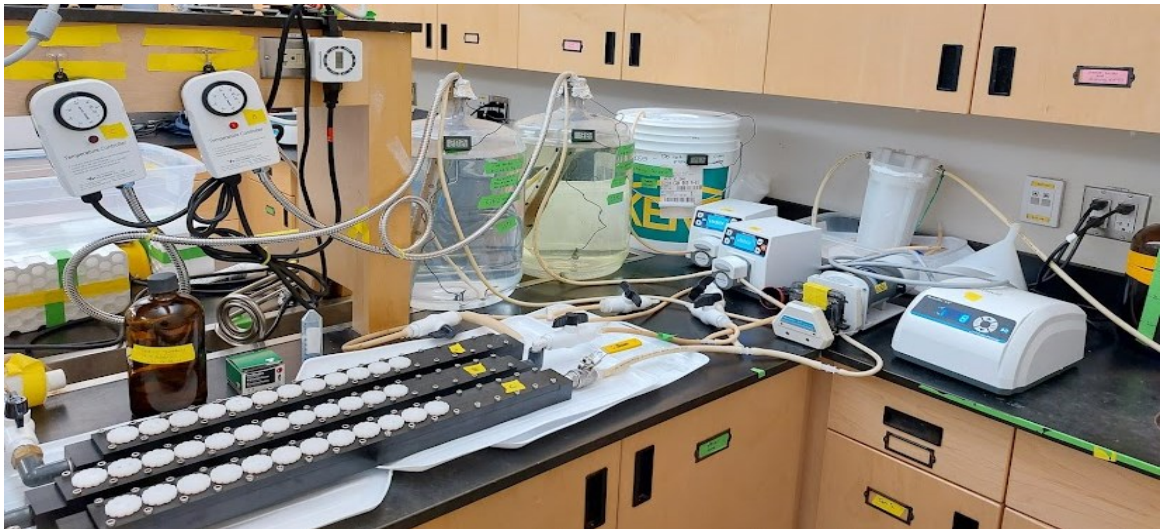
Figure 22. Biostud reactors (left) are connected in parallel with their feeding source (right). Experimental set-up.
