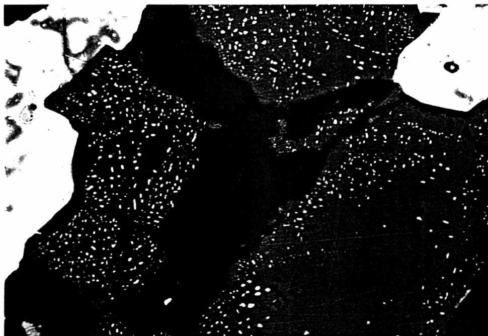
PHOTO 17: Exsolution blebs of chalcopyrite in sphalerite. (reflected light 250x)
