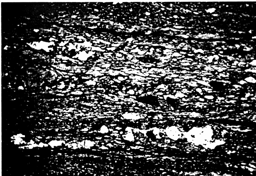
PHOTO 5: Stretched and oval augens in the porphyroclastic metavolcanics. (160x)
