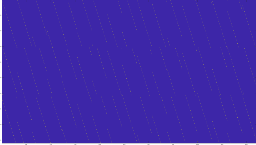
Figure 2.14: [5219, 4300] QC LDPC with \text{GF}(307) . With a = 9 , b = 17 , o(a) = 17 and o(b) = 3
