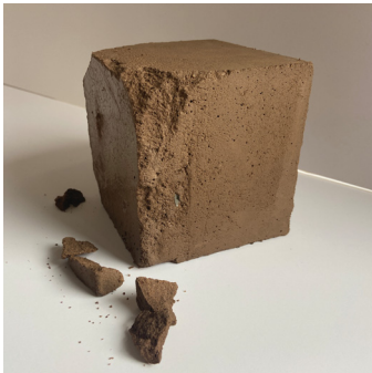
Mixture with clay used as aggregate
