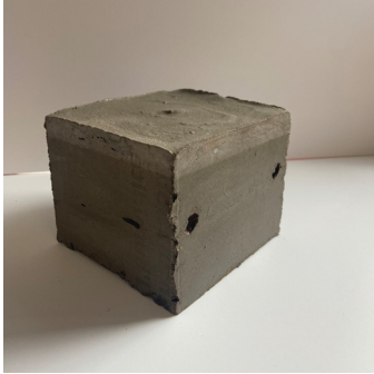
Mixture with chunks of clay throughout
