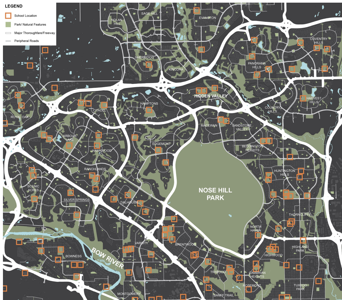
Diagram illustrating Calgary’s suburban neighbourhood unit typology. Each neighbourhood contains a school, natural features and parks, and are surrounded by perimeter roads for easy automobile access (The City of Calgary 2022).
