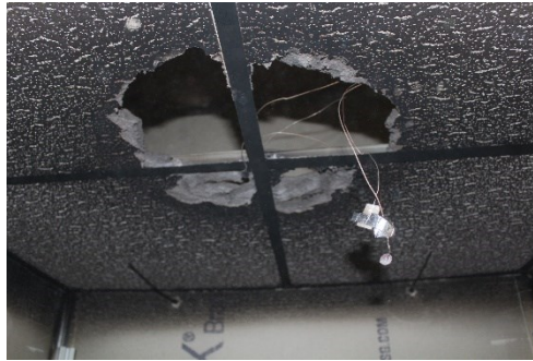
Figure 23 Endpoint condition of the NCTS from Test 2, with the delicate areas of the tile removed using minimal force by a pen.
