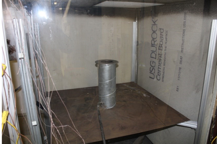
Figure 7 Adjustable platform surface and heat source within the apparatus.
