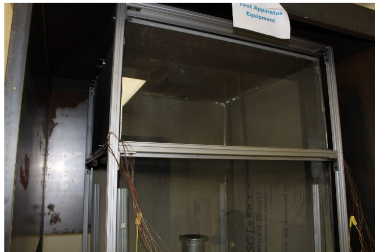
Figure 5 Testing apparatus frame and cavity space.
