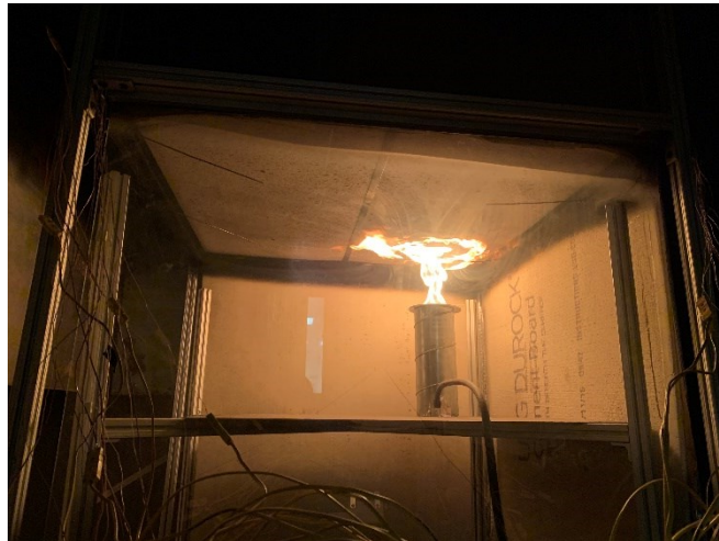
Figure 13 Propane burner in operation at a heat release rate of 13.5 kW with flame impingement on the ceiling tile system.
