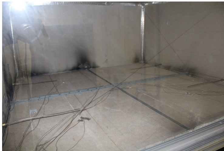
Figure 11 Cavity space above the ceiling tiles for an installed four-tile arrangement.
