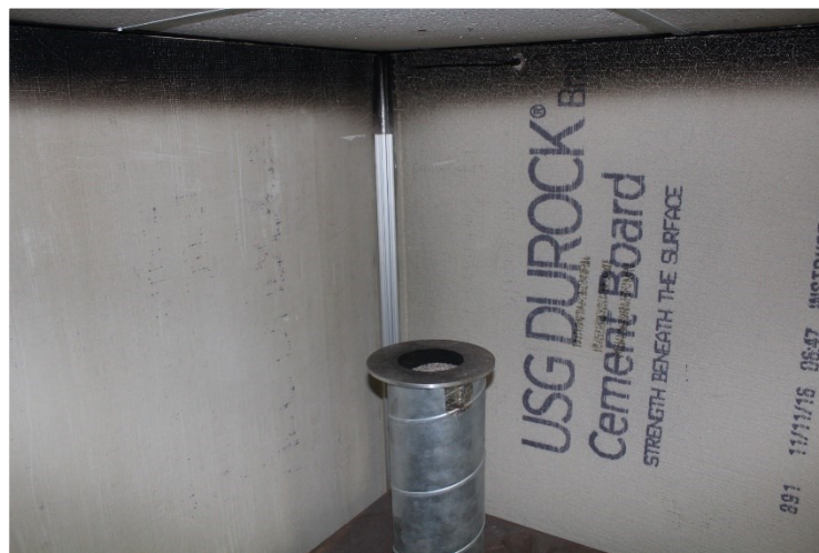
Figure 6 Cement board walls of the apparatus, as viewed from the interior.
