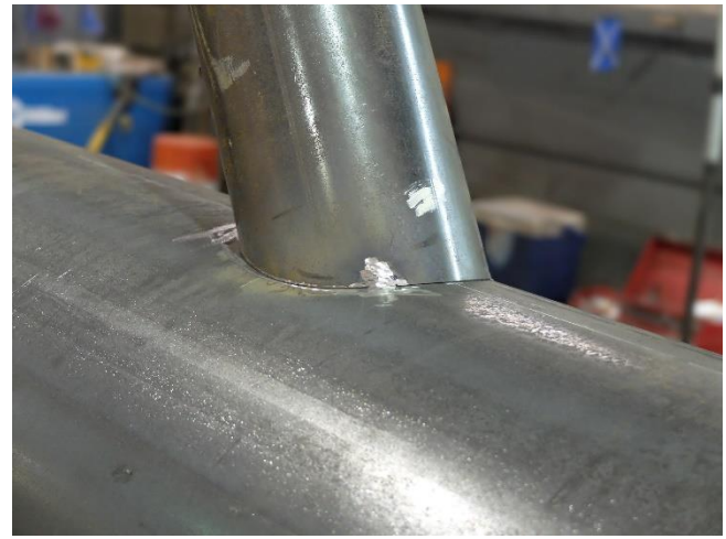
(b) Typical 60° connection (shown for 102-406-60b)
