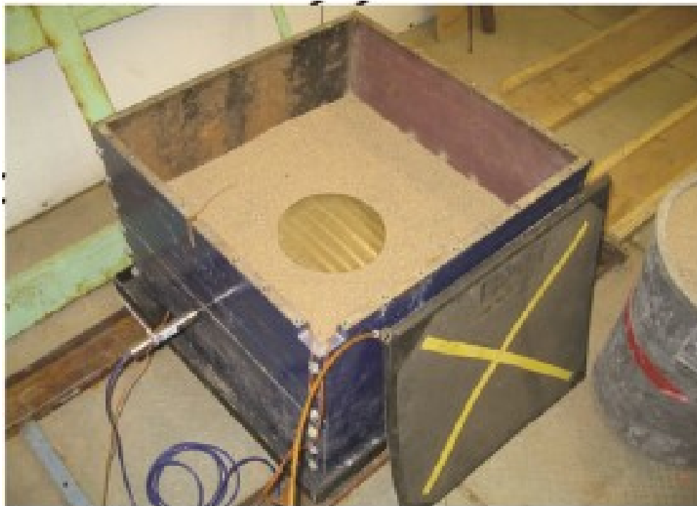
Figure 3.17: Pressure cell positioned in the pressure chamber (Huntley and Valsangkar, 2013).
