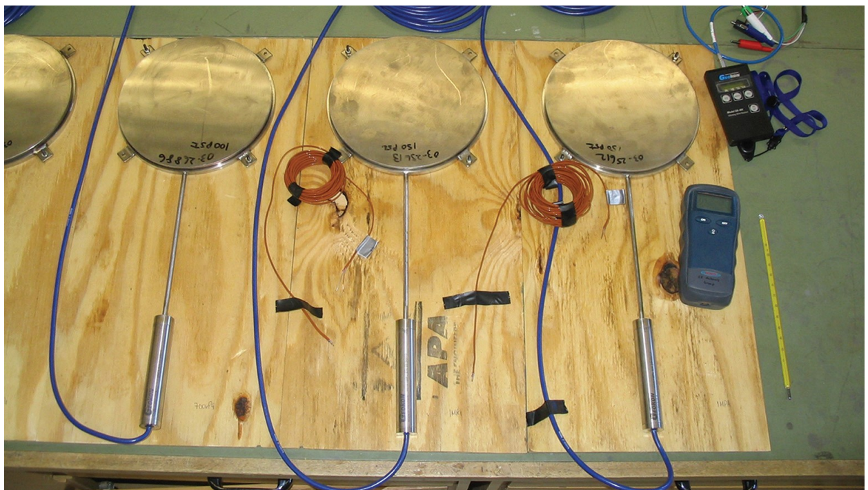
Figure 3.15: Contact pressure cells being tested in an unloaded state (Huntley and Valsangkar, 2013).
