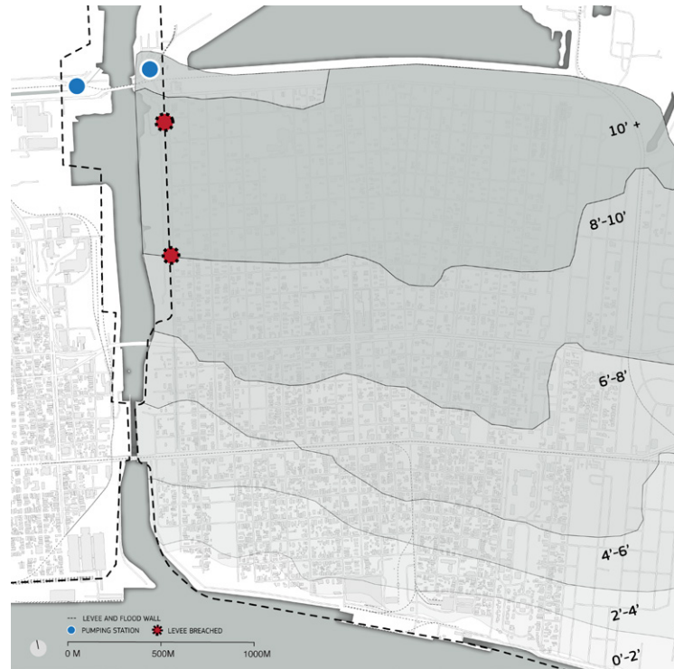
Diagram of the flooding after Hurricane Katrina in Lower Ninth Ward. (base map from Google Maps 2020; data from Swenson 2013; Waggoner and Ball 2013)
