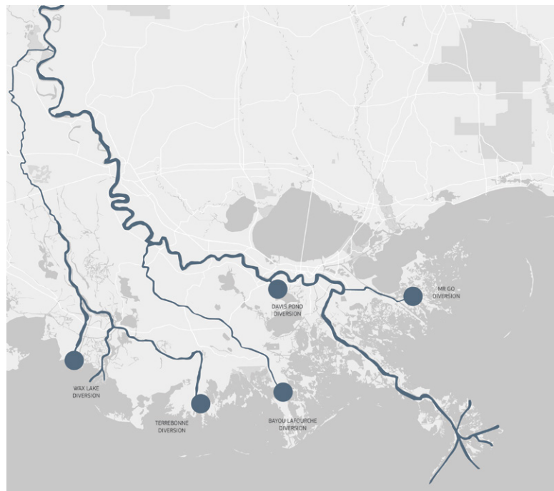
Diagram proposal of five diversion spillways to allow the Mississippi River Delta to return to its role as the delta builder. (base map from MapBox 2020; data from Mossop and Carney 2010)
