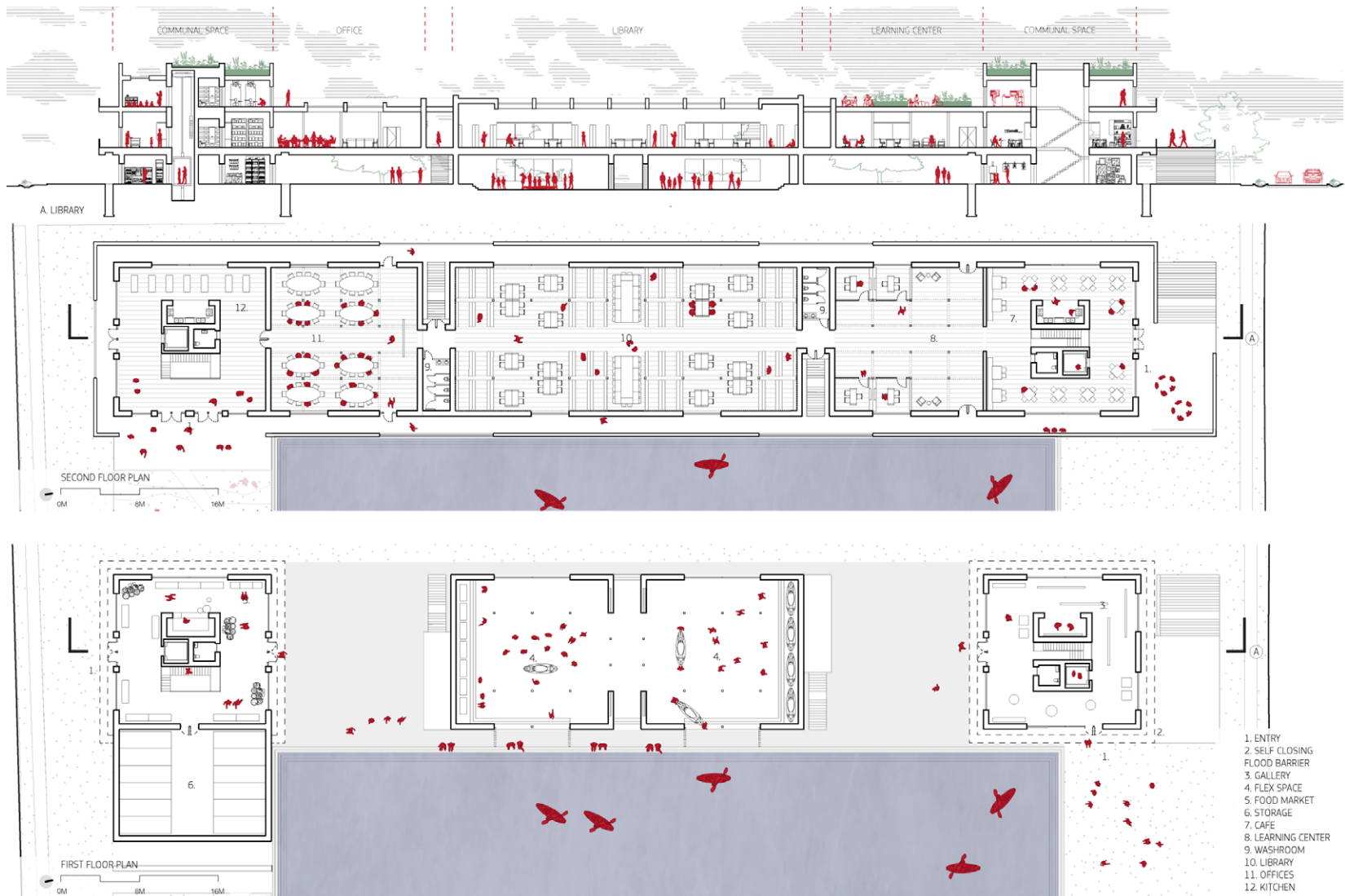
Section and plans show how spaces are used during the rainy season, where the plaza collects water for recreational use.
