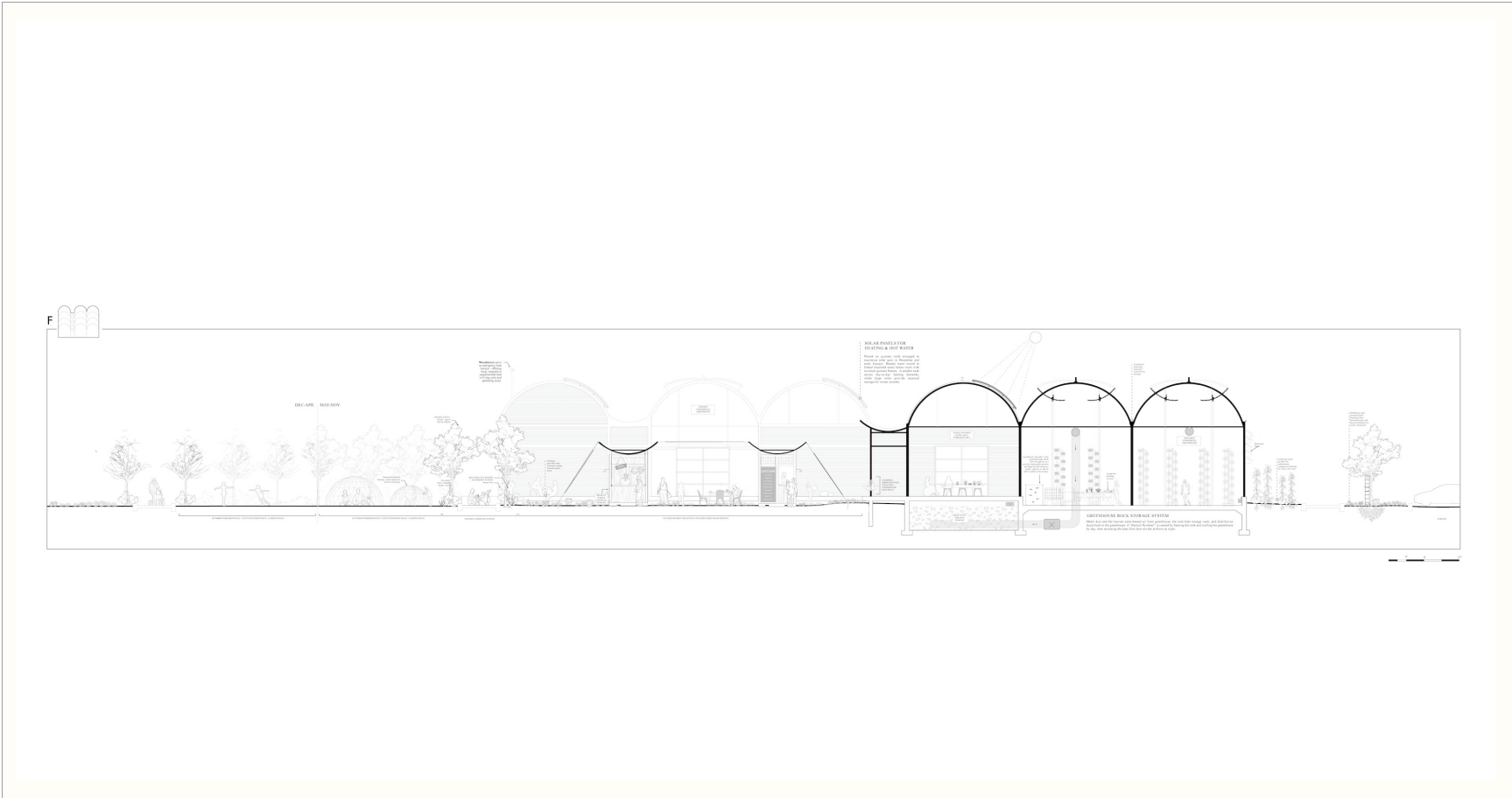
The section for the savant and learning center located at the south nucleus. The savant type, using the industrial gutter connected greenhouse frames, creates spaces for public programming demonstrated as a communal kitchen garden, market space which includes the shed type, covered eating and/or workshop area, and research greenhouses.
