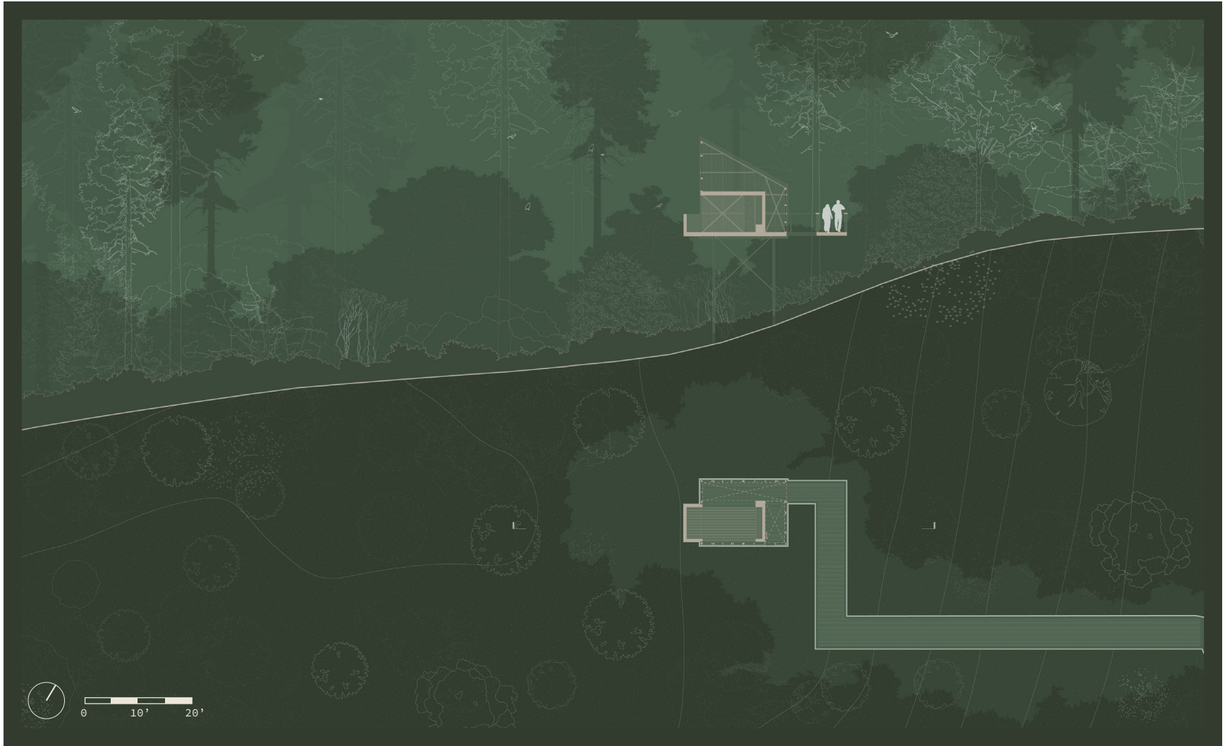
Birdwatch plan and section. Visitors start at grade in the forest floor and walk straight out into the forest understory.
