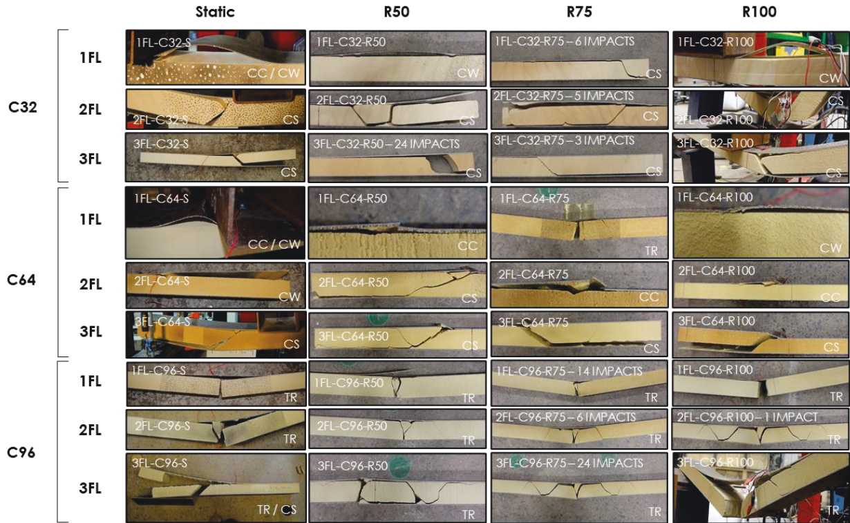
Figure 4. Failure modes of all specimens [Note static specimens were tested as a part of another study by Betts et al (2018)]
