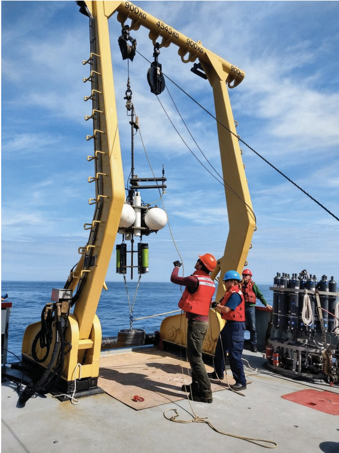
Figure 4: Hands-on, hanging deployment of the mooring from the aft A-Frame of CCGS Vector, demonstrating in-situ mooring orientation. The author is to the left. Aug 17, 2019
