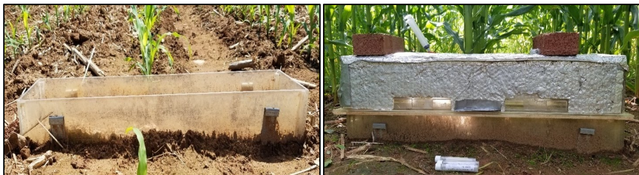
Figure 3.2: Installed collar in the field (left) and collar with the chamber on top during GHG sampling (right).
