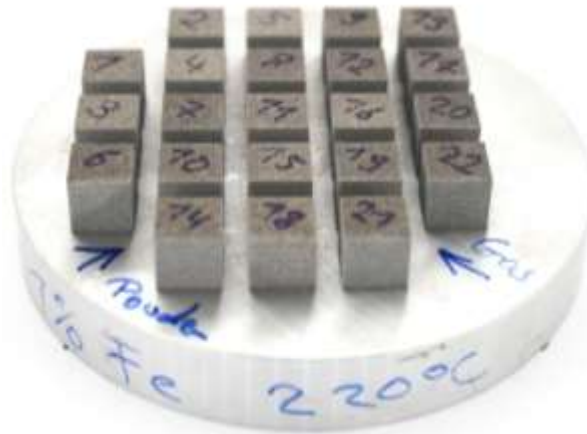
Figure 21. Solid ( 1\text{cm}^3 ) cubes produced using Al-1Fe powder.
