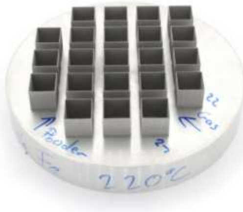
Figure 20. Image of single track hollow cube specimens produced with Al-1Fe powder.
