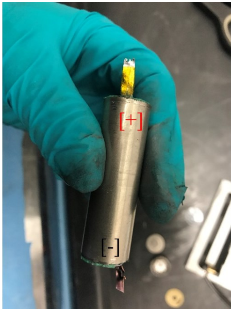
Figure 2.10 18-65 Base and top removed showing negative copper and positive aluminium current collector tabbing
