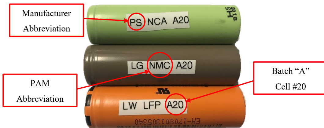
Figure 4.1 Panasonic NCR18650B (graphite||NCA), LG Chem ICR18650B4 (graphite||NMC) and Lithium Werks APR18650M1B (graphite||LFP). Scale 1:1
