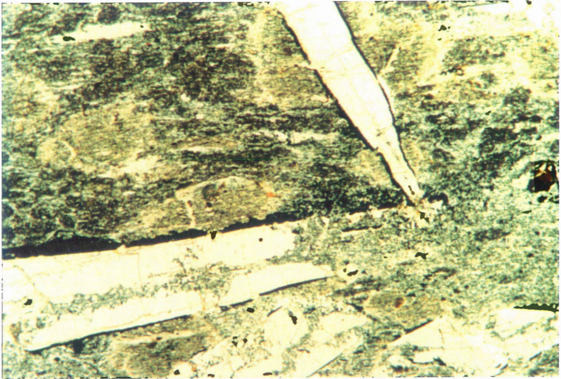
Fig. 4.5 Andalusite growing parallel and perpendicular to regional fabric (S1). Field of view is 3 x 5 mm.
