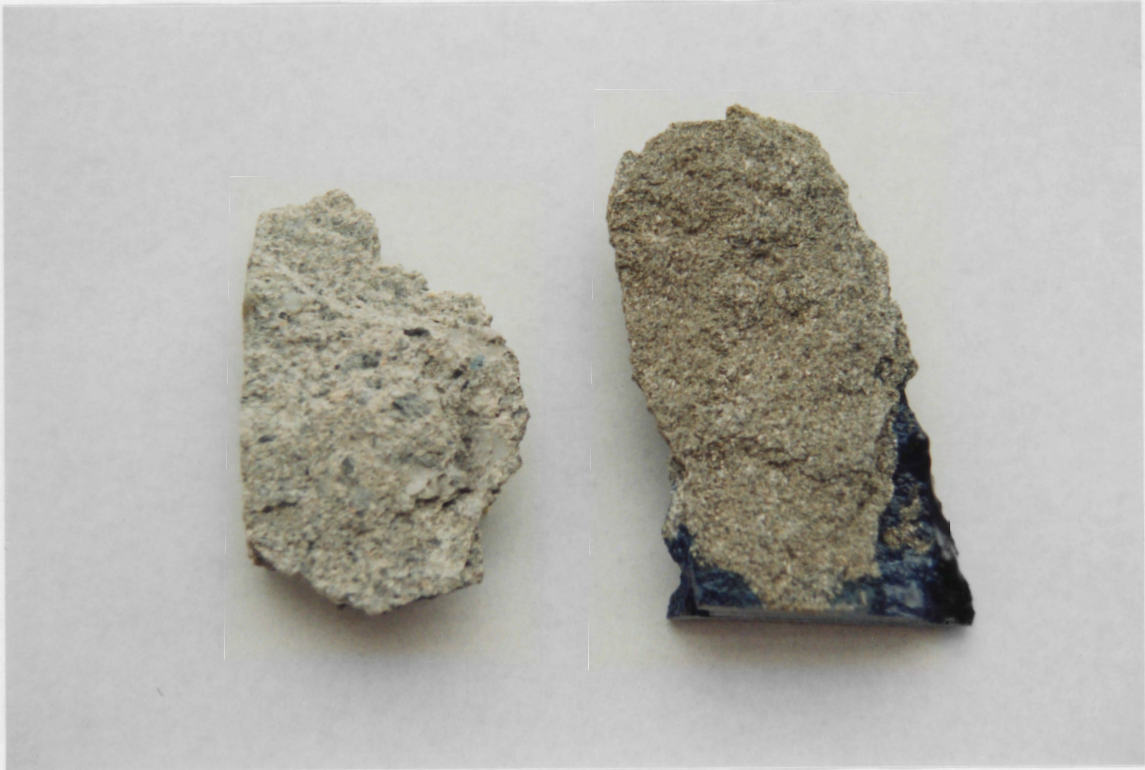
Figure 3.4 (B) Samples of OBT group. Sample on left of photograph is from Merlebach colliery, France. Sample on right is from the major Phalen outburst. Field of view is 22 cm.
