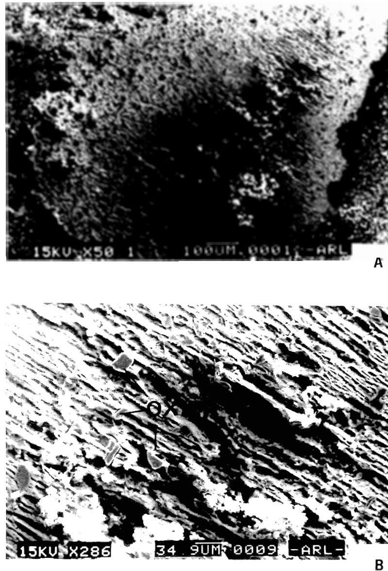
Figure 4.18: SEM images of anhedral pyrite in sample RJ-96-001 from the microbial treatment showing the surface after 42 days of oxidation. (a) An overview of the ridged anhedral pyrite grain surrounded by dark smooth matrix and with possible secondary minerals in the center (Fig. 4.20). (b) Deepest pit in the grain indicating very strong corrosion. Rounded oxide inclusions (ox) provide a baseline for topographic comparison, assuming the oxides have not changed and represent the level of the original polished surface. Ridges may be fine grey lamellae of the type seen in Figure 4.17.
