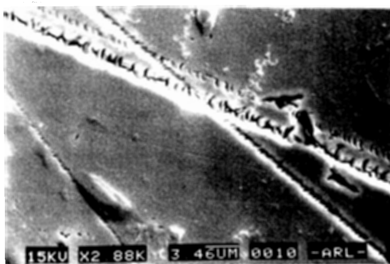
Figure 4.16: SEM image of sample RJ-96-001 from the microbial treatment showing etched polishing scratches in euhedral pyrite after 42 days of oxidation.
