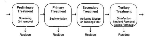
Figure 1 Municipal wastewater treatment levels ranging from preliminary, primary, secondary, and tertiary levels of treatment. Leftover residues from each treatment is called "sludge" (National Research Council, 1996).
