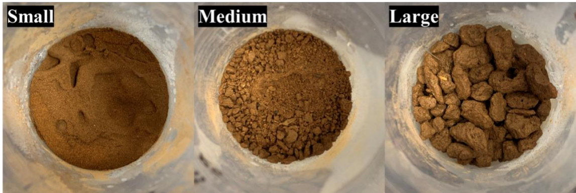
Figure 2: Twenty-five gram of soil air-dry equivalent placed in 100 mL DigiTube plastic vials, including three aggregate size fractions: 0 to 0.25 mm (small), 0.25 to 4 mm (medium), and 4 to 8 mm (large).
