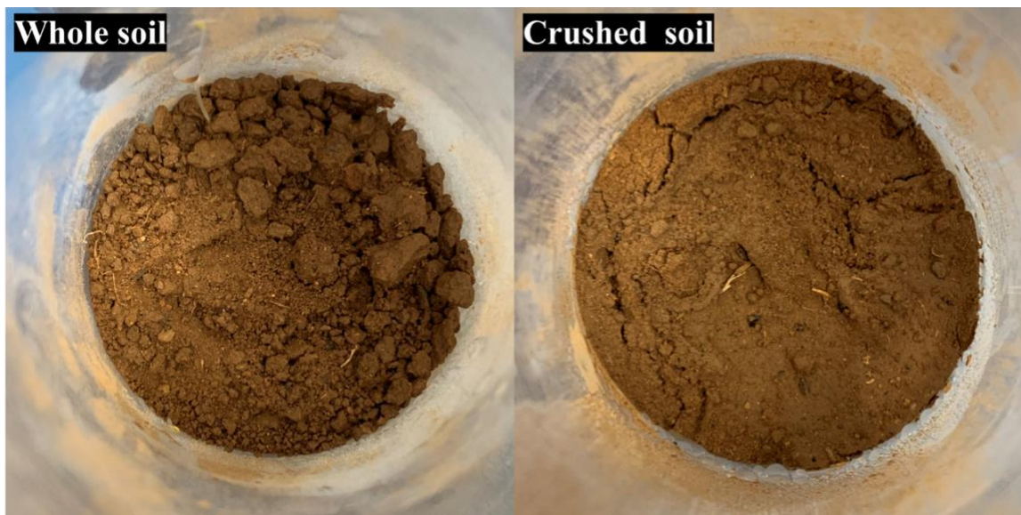
Figure 1: Twenty-five gram of soil air-dry equivalent placed in 100 mL DigiTube plastic vials, including the soil presence of aggregate (whole soil) and the soil in which the aggregates have been crushed (crushed soil).
