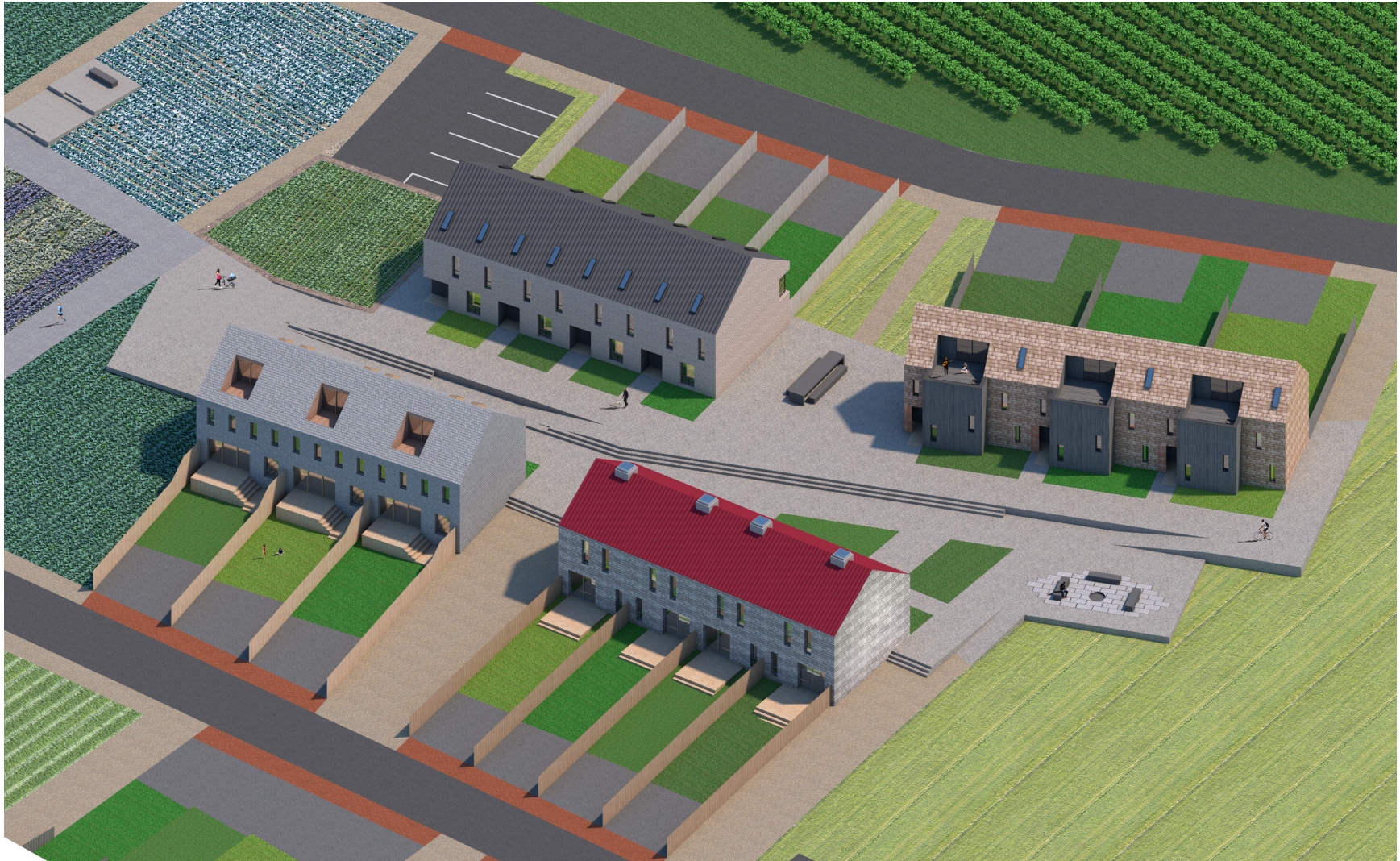
Neighbourhood cluster axonometric drawing highlighting relationship between private yards, public growing spaces and pedestrian network.
