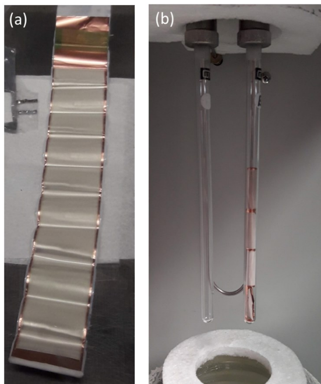
Figure 2-6. (a) Negative electrode with plated lithium metal after charging in an anode-free lithium-metal pouch cell. The electrode is ~40 cm long. (b) Electrode cut into four pieces and loaded into BET tube for surface area measurement.
