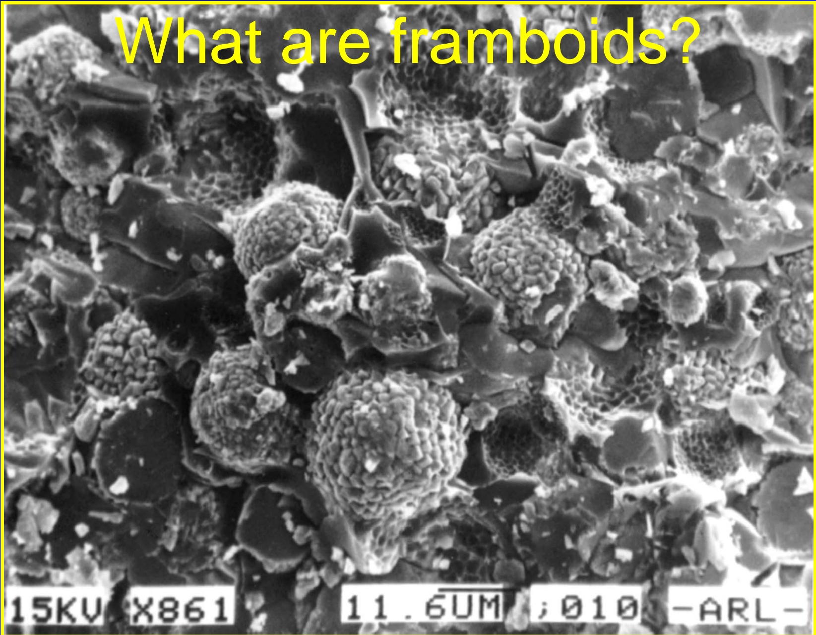
Scanning electron microscope (SEM) image of pyrite framboids (Wilson, 1998)
