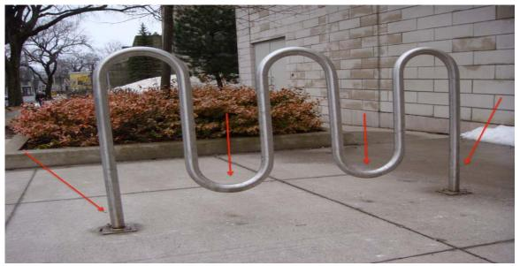
Figure 1: An example of a typical wave rack. The red arrows indicate spots where the researchers assumed that one bicycle could be stored. Thus, for all wave racks the capacity was determined by counting the end posts and the dips in the wave.
