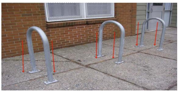
Figure 3: An example of typical staple racks. The red arrows indicate spots where the researchers assumed that one bicycle could be stored. Thus, for all staple racks the capacity was determined by assuming that each inverted-U could support two bikes.
