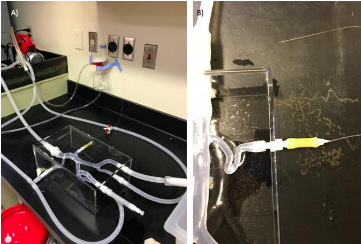
Figure 4.2: A) Complete setup of the benchtop model, B) stepwise reduction from the 'renal artery' to the 'arteriole' to the capillary bed.
