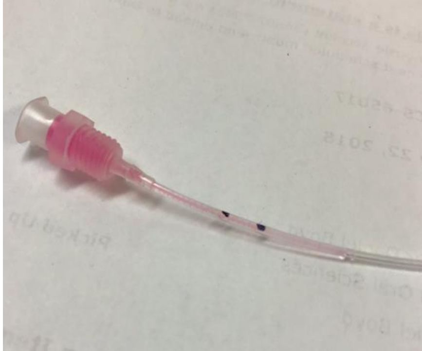
Figure 4.3: Reduction adaptor and micro-tubing filled with EmboSphere® suspended in DMEM following completion of one trial.
